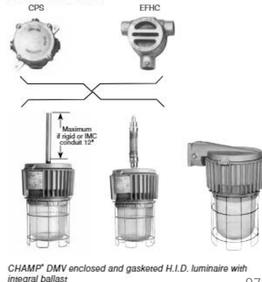
Pendant Fixtures and Supports, Class II. Suggested Installation Methods
